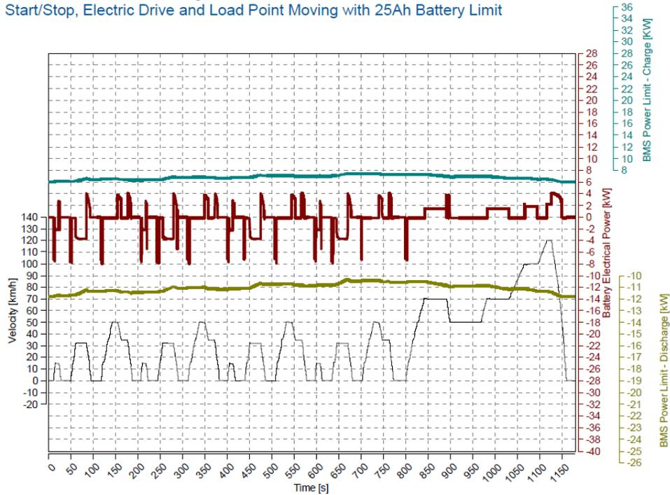
Figure 7. Battery power, BMS charge and discharge limits and velocity profile with a 25 Ah battery, ALABC project 1012N with AVL Schrick GmbH, 2012.
