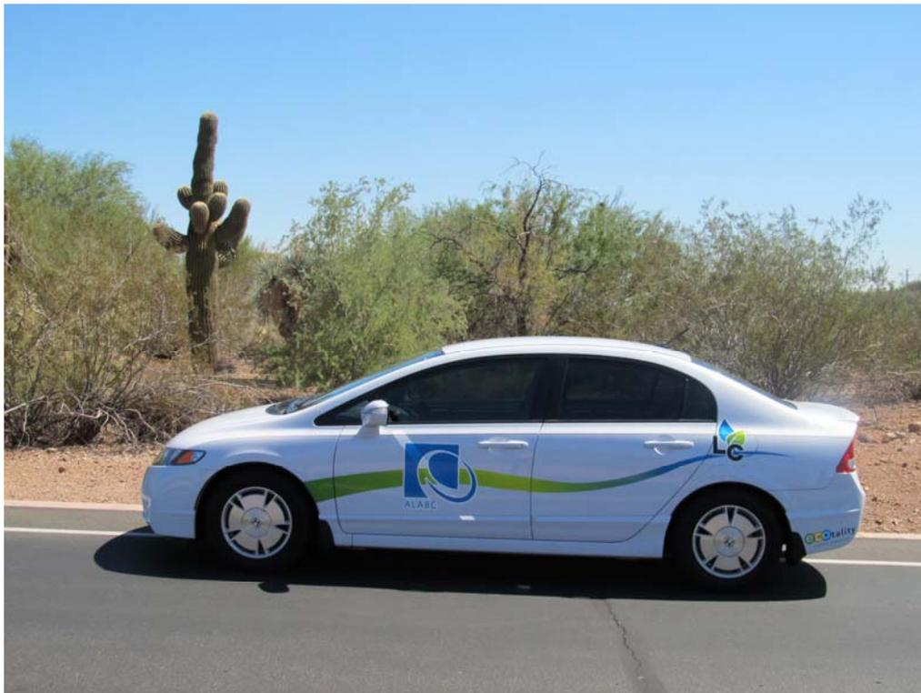
*Figure 4. The Honda Civic in which the original nickel - metal hydride battery has been replaced with an ‘UltraBattery’.*
