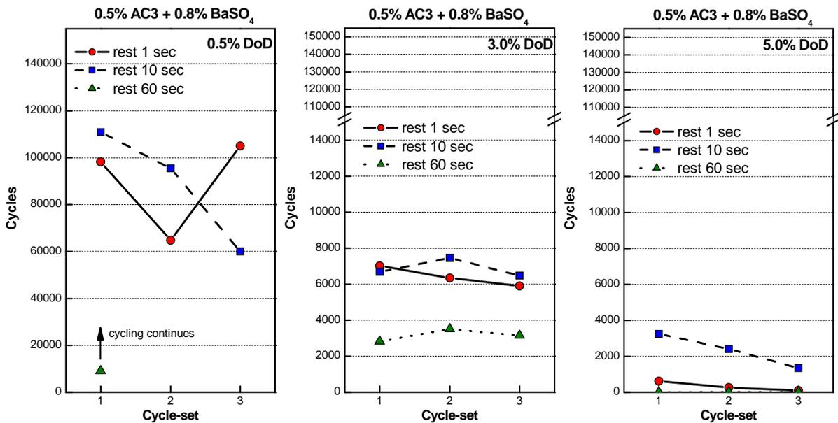
Figure 8. Cycling plots of cells with same additives at three DOD levels and three rest times, ALABC project 1012G with the Bulgarian Academy of Sciences.
