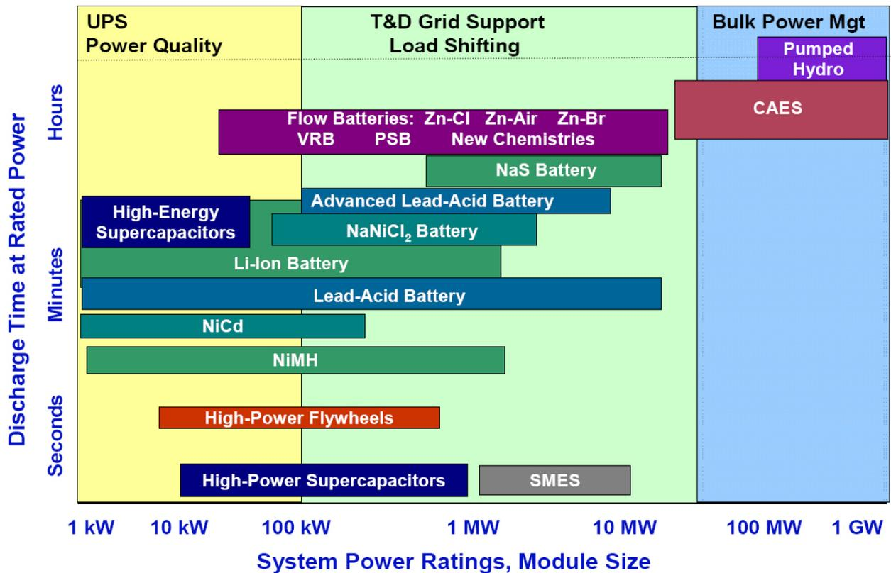
Figure 6. Positioning of Energy Storage Technologies (Source EPRI primer - Electric Energy Storage Technology Options, December 2010)
