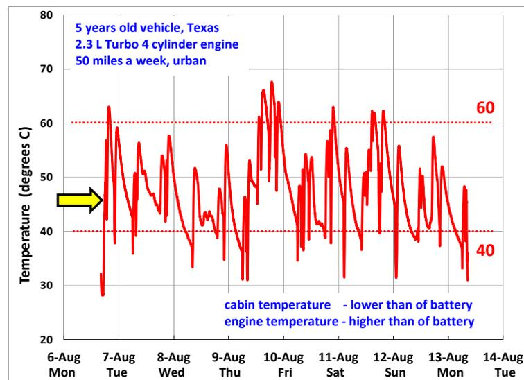
Figure 9. Battery temperatures in an 'average' vehicle used in city traffic in Texas (courtesy of Dr. J. Hohn, RSR).
