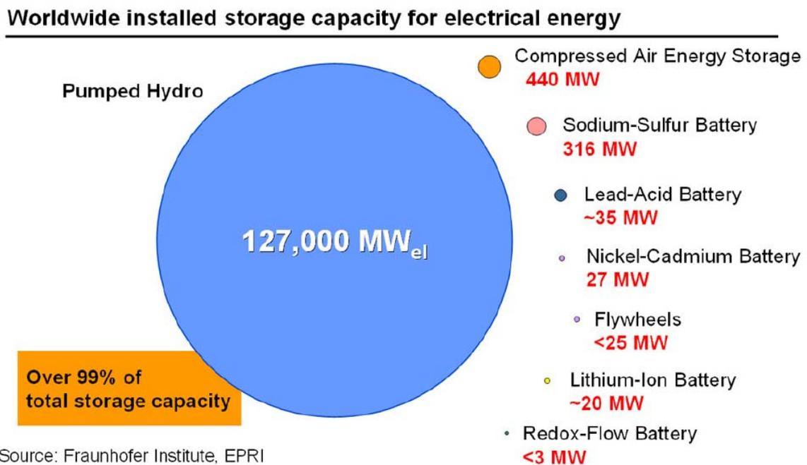
Figure 5. Worldwide Installed Storage Capacity for Electrical Energy (Source EPRI primer -Electric Energy Storage Technology Options, December 2010)
